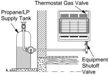
Figure 18 - Checking Gas Joints for Propane/LP Gas
